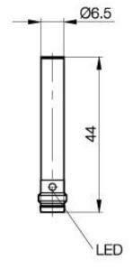
Inductive Sensors BES 516-372-G-E5-C-S 49 D6.5 x 44 normally-open Sn=2mm shielded
